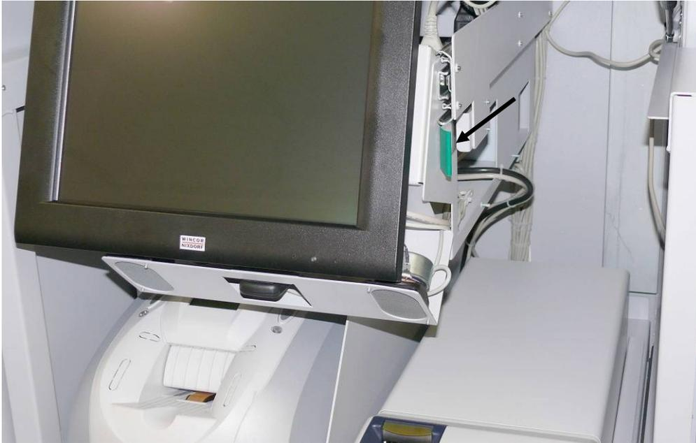
The power supply unit is located on the carrier underneath the keyboard.
