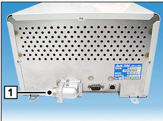
Check that the connector (1) is correctly inserted on the rear of iCash 15.
