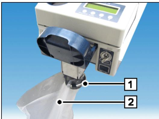
Lift the ring at the base of the safe bag holder (1), attach the safe bag (2) and press the ring down again.
