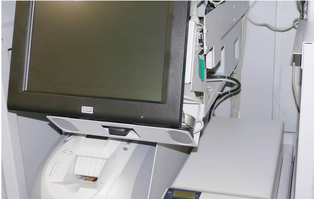
The special electronic module is fixed on the bottom side of the carrier of the touchscreen.
