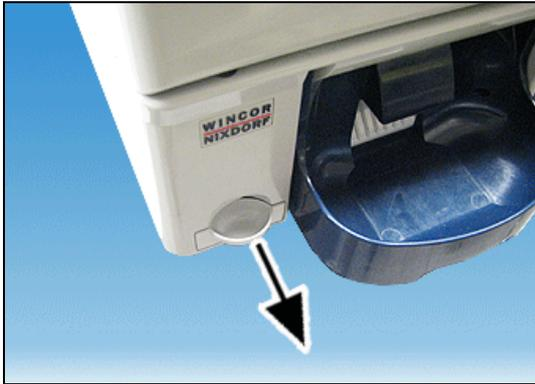
Pull the dust box (1) out of the device.
