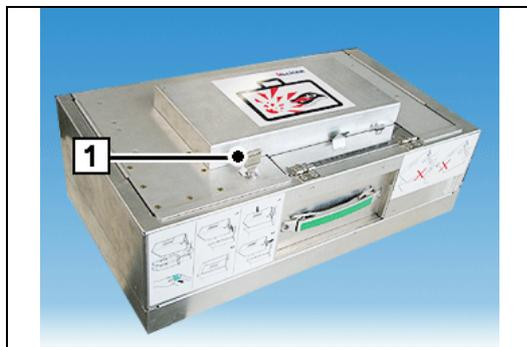
When you have pressed a key, the stacker cassette displays its current status via LEDs that blink in the IR window (1) for approx. 5 seconds (see section "Signals issued by the stacker cassette").
