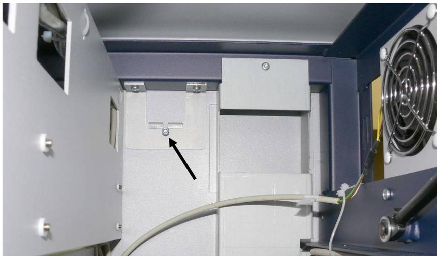
After setting the back panel in place, do not forget to fix it with the screw from inside again.
