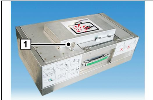
The stacker cassette indicates its current status in response to a status query (see section "Querying the status of the stacker cassette") via LEDs that blink in the IR window (1).
