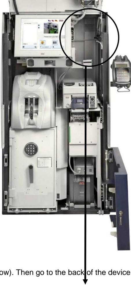
Remove the screw (arrow). Then go to the back of the device and remove the back panel upwards.
