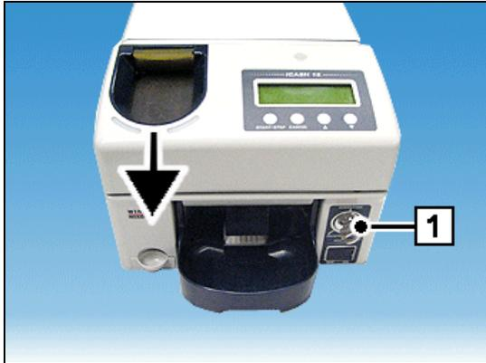
Insert the key in the lock (1), turn it as far as possible to the right and hold it in this position.
